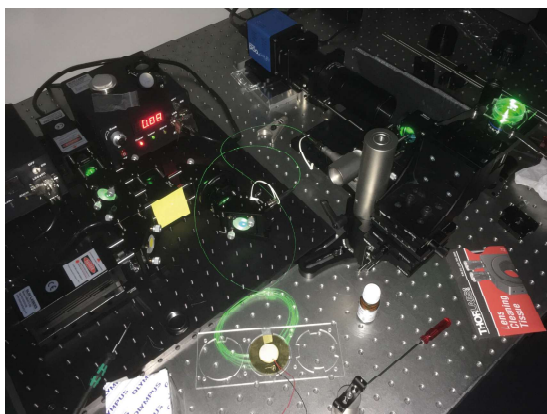
Two-colors total internal reflection fluorescence microscope (TIRFM) for single molecule FRET currently in development in the Dulin lab.
